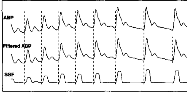
Figure 2-6: Beat extraction based on wabp . The SSF function amplifies the rising portion of each beat. Adapted from [43].
