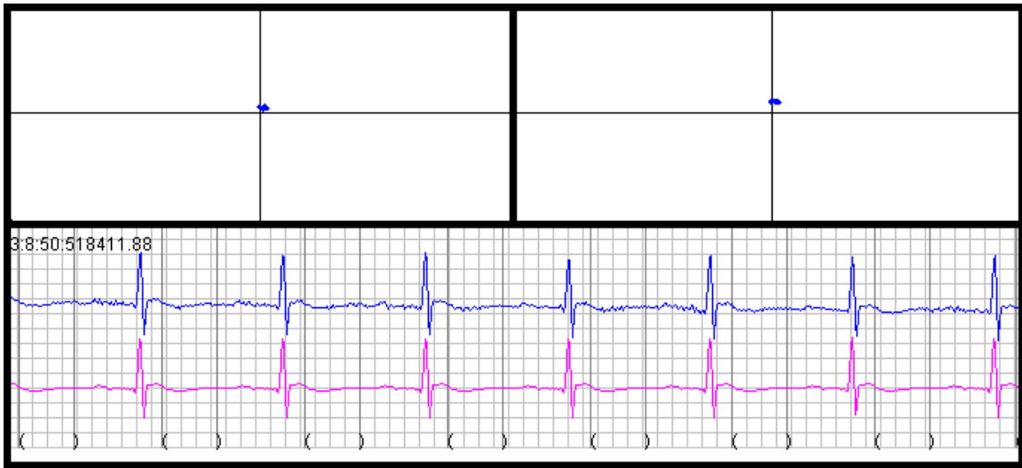
Figure E-20: Chebyshev decomposition example 20 of 23 - the top-left scatter plot shows approximately 100 consecutive data points (beats) of Chebyshev coefficient 1 (slope) vs. Chebyshev coefficient 0 (offset relative to isoelectric value); the top-right scatter plot shows Chebyshev coefficient 2 (curvature) vs. Chebyshev coefficient 0; the lower plot shows the underlying ECG waveform, where the top signal is the raw waveform and the bottom signal is a 64-beat trailing average beat.
