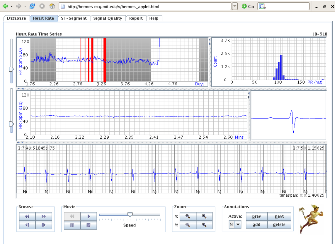
Figure C-3: In this example the user has selected a memory depth of 5 to recall previously visited points of interest in the long-term heart rate trend plot. The thickening bars from left to right indicate that the user is navigating from left to right.
