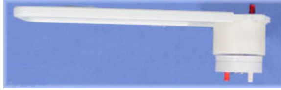
Figure 1-5: One cable (not shown) connects this commutator to the terminal point of the tripolar leads (fig. 1-4). Another cable (not shown) connects this commutator to the input of the analog instrumentation (discussed in chapter 3). The commutator swivels freely and thus permits the subject to move uninhibited and without tangling lead wires.
