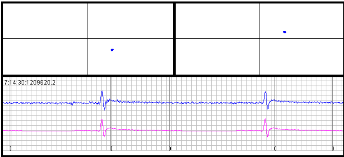
Figure E-3: Chebyshev decomposition example 3 of 23 - the top-left scatter plot shows approximately 100 consecutive data points (beats) of Chebyshev coefficient 1 (slope) vs. Chebyshev coefficient 0 (offset relative to isoelectric value); the top-right scatter plot shows Chebyshev coefficient 2 (curvature) vs. Chebyshev coefficient 0; the lower plot shows the underlying ECG waveform, where the top signal is the raw waveform and the bottom signal is a 64-beat trailing average beat.
