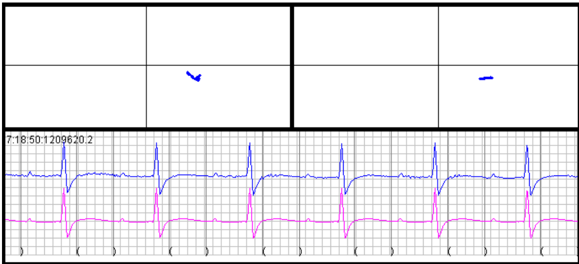
Figure E-15: Chebyshev decomposition example 15 of 23 - the top-left scatter plot shows approximately 100 consecutive data points (beats) of Chebyshev coefficient 1 (slope) vs. Chebyshev coefficient 0 (offset relative to isoelectric value); the top-right scatter plot shows Chebyshev coefficient 2 (curvature) vs. Chebyshev coefficient 0; the lower plot shows the underlying ECG waveform, where the top signal is the raw waveform and the bottom signal is a 64-beat trailing average beat.
