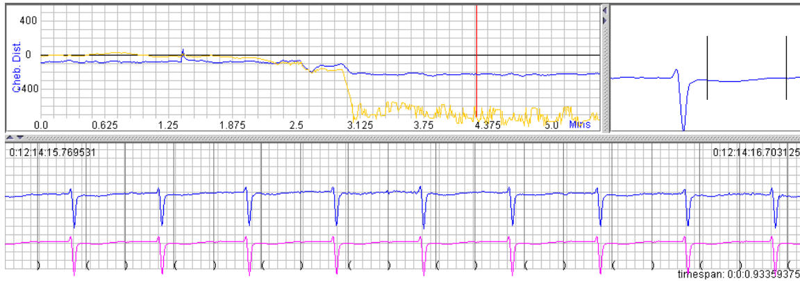
Figure 6-8: The upper-left panel shows the blue repolarization metric time series (signed Euclidean morphology metric, which remains closer to zero after 3.125 minutes than the other signal) and the yellow QRS integral time series (to be discussed in upcoming sections); the upper-right panel shows a 64-beat trailing average beat with repolarization period time markers (vertical bars); the lower panel shows the original ECG waveform time series (upper signal) and the 64-beat trailing average waveform time series. The placement of the vertical bar in the upper-left panel indicates that the waveform data in the other panels corresponds to a point in time after a substantial change in the repolarization metric from approximately -100 at 2.5 minutes to approximately -200 at 3.125 minutes. Inspection of QRS morphology and the rapidity of its change indicate a probable axis shift from subject movement.
