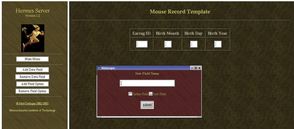
Figure 4-5: In this screenshot the user is adding a field entry to the default mouse record template. Note that the field can be of type “text” or of type “option.” If the field is of type “text,” then the user can freely type alphanumeric characters (enforced by a JavaScript routine) when creating the mouse record. If the field is of type “option,” then the user will select one of several pre-defined mutually exclusive options from which to select in the mouse record. Defining the options themselves for a given field is done in a manner similar to that of adding a field.
